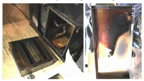
(2) The Baffle filter and the tray in C-Box should be washed with soap and warm water in every week.
